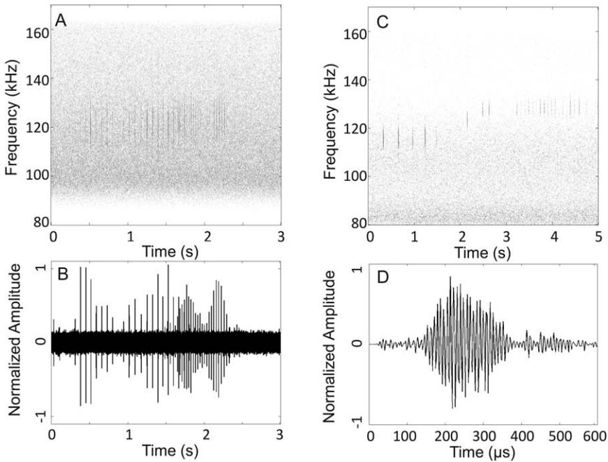
Figure 2. Examples of the burst-pulse clicks (A, B) and the lower frequency clicks (C, D) from Guam, including an example spectrogram (A) and time series (B) of the burst-pulse clicks, and an example spectrogram (C) and waveform (D) of the lower frequency clicks. The burst-pulse is visible in A and B between 1.6 s and 2.4 s. Lower frequency clicks are visible in C between 0 s and 1.5 s, followed by usual clicks from 2.5 s to 5 s.
